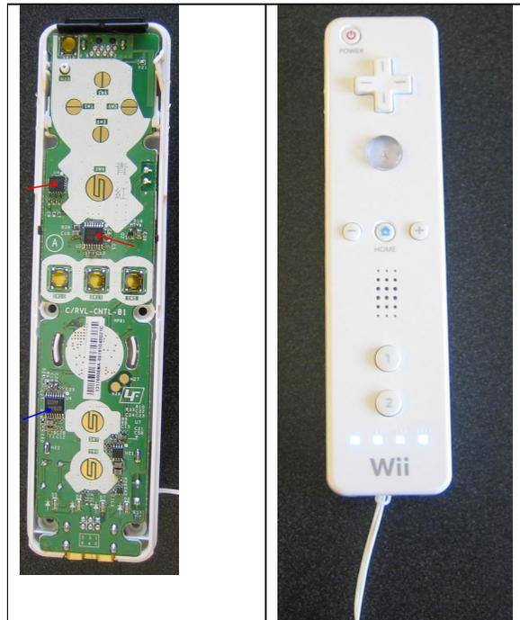
On this picture we can see a wii mote joystick based on a Bluetooth radio and a three axes accelerometer, which is considered the primary reason for the success of the video game.
